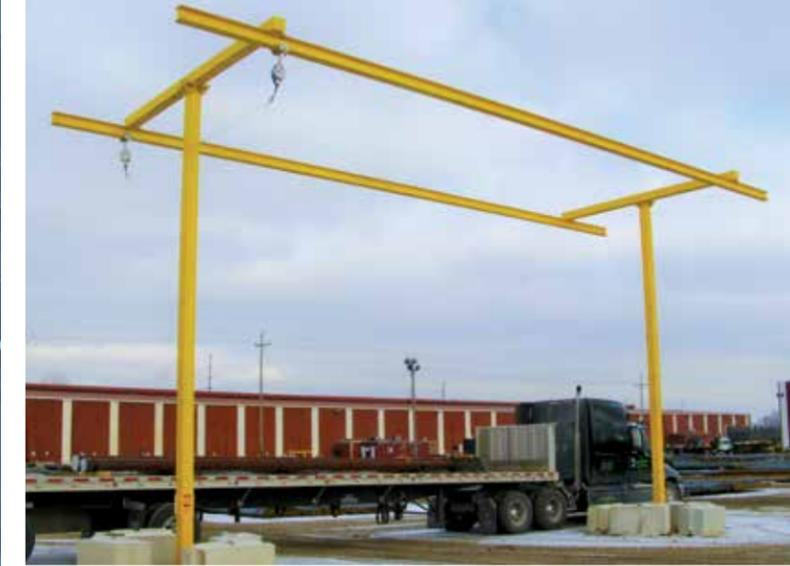
There are two very important design considerations when determining your gallows system. The height of your railcars or trucks establishes your fall clearance, this in turn determines if a rigid or cable system can be used. Also, it is important to know the soil compaction around your tracks so the foundations of the gallows can be designed correctly.
